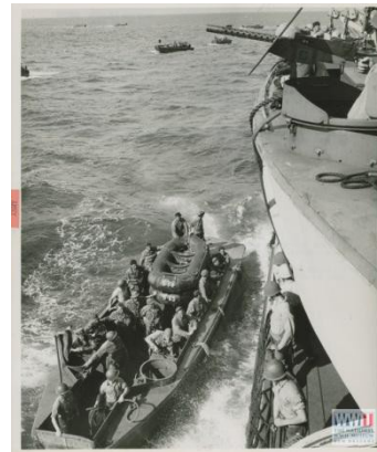
Special operations troops departing their mother ship in an LCPR, with their rubber boats stacked on the stern
